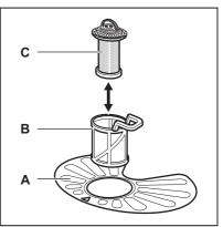
1. Turn the filter (B) counterclockwise and remove it.
