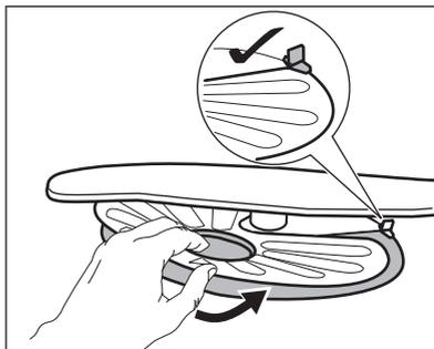
7. Reassemble the filters (B) and (C).
