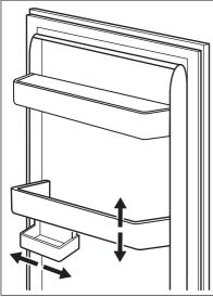
This model is equipped with a variable storage box which can be moved sideways.
