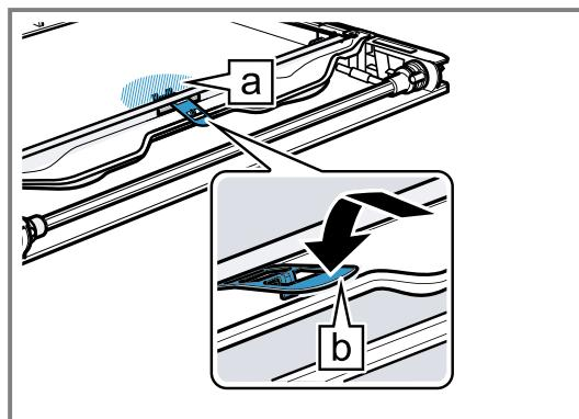
7. Place the inner pane onto the appliance door so that the number **a** is legible at the bottom right. Insert the inner pane into the fixing rail **b** at an angle towards the back.
