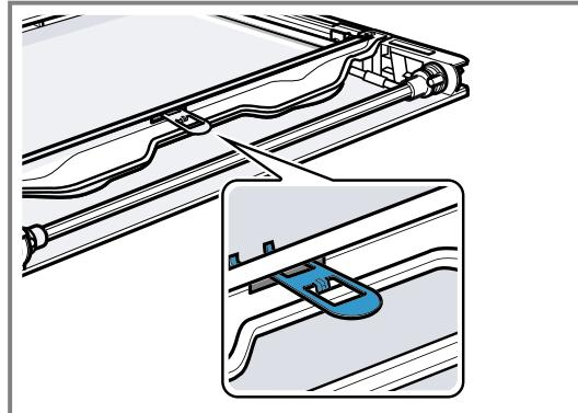
✓ The retainer has been inserted.
