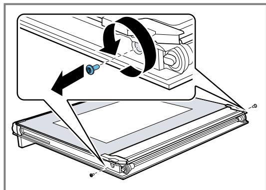
3. Carefully lift the inner pane upwards at an angle ① and remove the holder ②.
