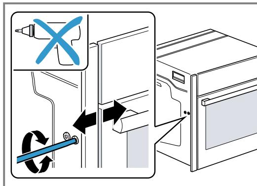
Turning the screws clockwise makes the gap larger
