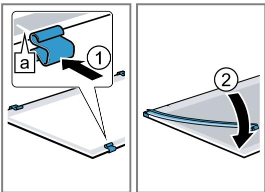
4. Insert the intermediate pane with spacers and seals in the direction of the arrow ①.
