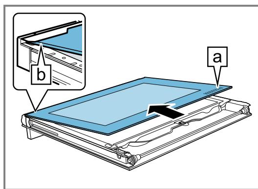
8. Carefully lift the inner pane upwards at an angle and attach the holder **a**.
