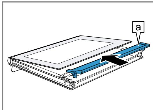
9. Insert the inner pane with the holder **a** into the opening.
