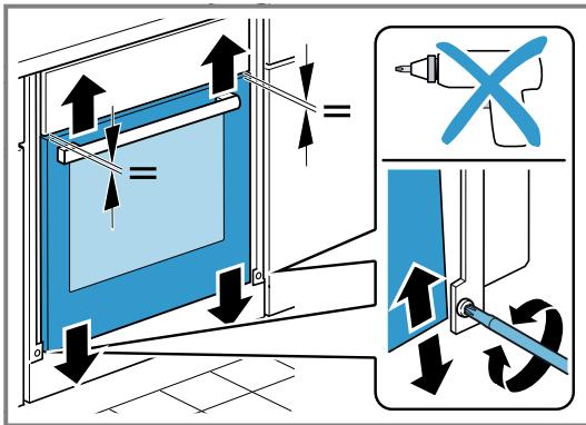
Turning the screws clockwise makes the gap smaller
