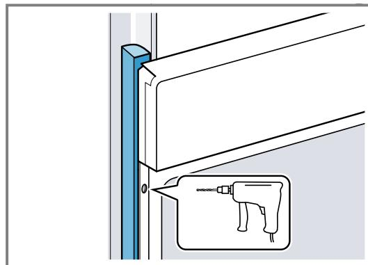
4. Secure the appliance using a suitable screw.
