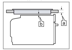
The minimum worktop thickness **b** is based on the required minimum clearance **a**.
