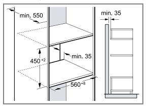
To ventilate the appliances, the intermediate floor must have a ventilation cut-out.
