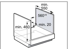
To ventilate the appliance, the intermediate floor must have a ventilation cut-out.
