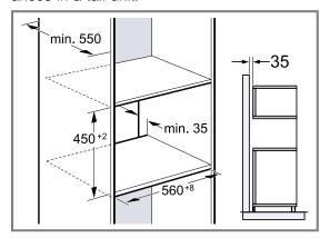
To ventilate the appliance, the intermediate floor must have a ventilation cut-out.
