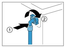
2. Connect the water inlet hose to a tap (26.4 mm = 3/4").
