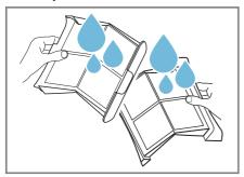
Note: Collect the cleaning water in a container, e.g. a bucket. After cleaning, pour the contents of the container through a filter, e.g. a coffee filter.
