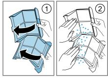
Dispose of the fluff with the household waste in order to prevent the water from being contaminated with microplastics. **6.** Clean the two fluff filters thoroughly under warm, running water and then dry them off.
