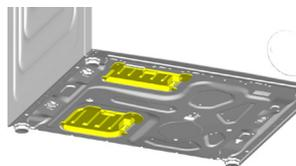
Rest the tabs of Cover B against the lower panel. Complete the assembly by rotating the cover.
