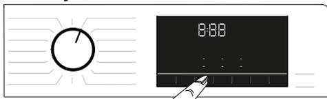
Select the desired auxiliary functions before starting the programme. Whenever a programme is selected, icons of the auxiliary function symbol that is selected together with it illuminates.
