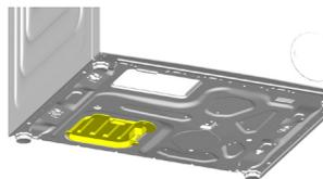
Tilt the machine back slightly. Rest the tabs of Cover A against the lower panel. Complete the assembly by rotating the cover.
