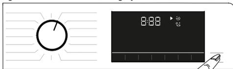
If the water level in the machine is not suitable when you press **Start/Pause** button, the door lock cannot be deactivated and the door lock icon on the display remains on.
