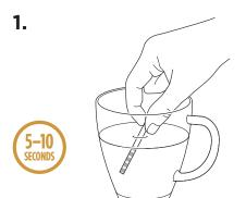
Locate test strip provided in starter kit. Completely submerge test strip in the water you plan on using with your machine for 5-10 seconds, ensuring all squares are underwater.
