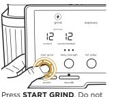
Press **START GRIND**. Do not touch portafilter until grinding is complete.
