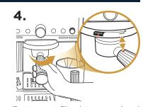
Fasten portafilter into group head until orange dot on portafilter aligns with lock arrow on group
