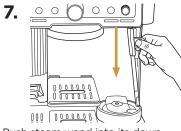
Push steam wand into its down position. The machine will automatically purge to clean inside of wand.
