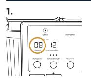
Check to see if the current grind setting matches the recommended setting.
