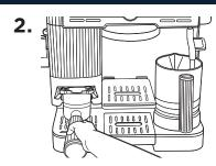
Release the tamper lever and remove the portafilter from the grinding cradle.
