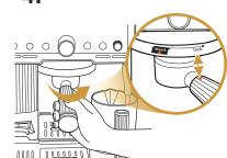
Fasten portafilter into group head until orange dot on portafilter aligns with lock arrow on group head.
