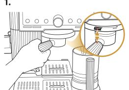
With the double basket installed in the portafilter, place the portafilter in group head (angled to the left) by aligning orange dot on portafilter with orange dot on group head.
