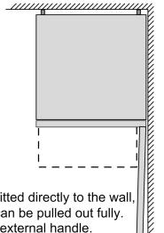
If the appliance is fitted directly to the wall, all of the drawers can be pulled out fully.
