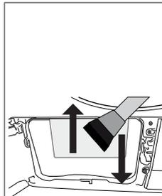
Clean the fibre on the metal surface of the condenser with damp cloth or the brush on the air deflector in up - down direction. Do not clean with left - right direction since it will damage the metal plates of the condenser.
