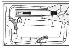
After cleaning the filter, door and the condenser, drag the brush to the right and lock it in its place.
