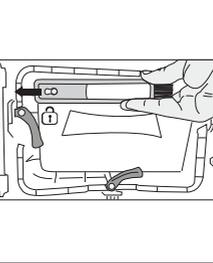
Pull the brush to the left to remove it. You can use the cleaning brush to clean lint filter, condensing metal surface and accumulated fibre on the door.
