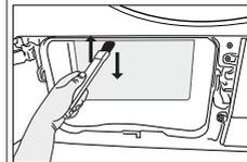
You can use a vacuum cleaner with a brush for cleaning. If the vacuum cleaner does not have a brush, it is not recommended to be used for condenser cleaning.
