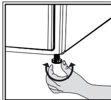
Until the drying machine stands level and sturdy, adjust the stands by turning them left and right.
