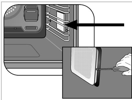
3. Lift the lamp's protective glass cover with a screwdriver.
