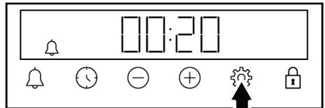
⇒ After setting the alarm time, the
