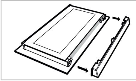
3. As shown in the figure, gently lift the innermost glass (1) towards “A” and then, remove it by pulling towards “B”.
