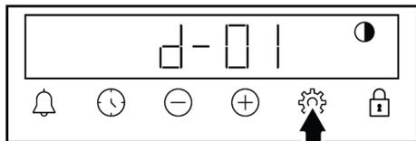
2. Set the desired brightness with the ⊕/⊖ keys. (d-01-d-02-d-03)
