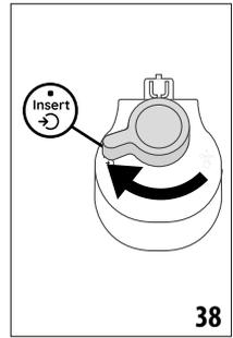
3. Turn the froth adjustment dial (E3) or (F3) clockwise to the "Insert" position (fig. 38) and pull to extract;
