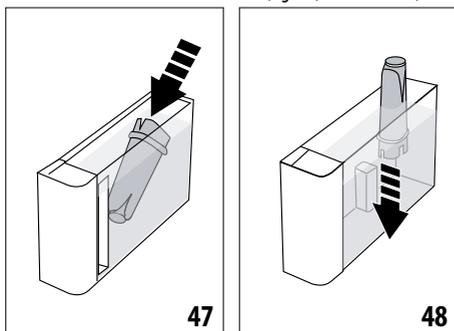
7. Extract the water tank (A22) (fig. 2) and fill with water; insert the filter in the water tank and immerse it completely for about ten seconds, sloping it and pressing it lightly to enable the air bubbles to escape (fig. 47). Press "Next";
