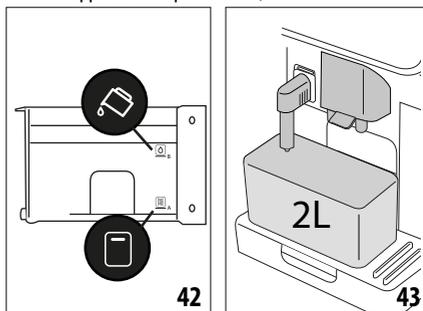
9. Place an empty 2 litre container under the spouts (fig. 43). Press "Next" to start descaling ("Back" to go back to the previous screen or "X" to exit the procedure, remembering to remove the descaling solution from the tank)
