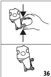
9. Once inserted, make sure the two coloured buttons have snapped out;
