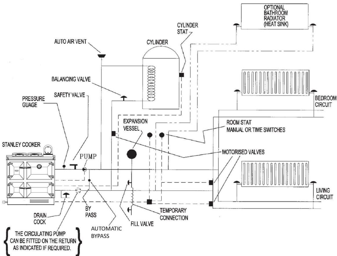
**OPEN SYSTEM (WITH PUMP ON FLOW)**
