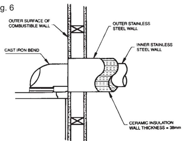
Where the flue passes through a combustible material, a twin wall solid packed insulated chimney connector must be used and must come flush with the outer surface of the material and run all the way to the masonry chimney or to the point of termination of the factory-made chimney. (See Fig.6)
