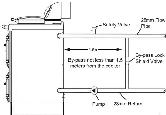
A 15mm system by-pass must be fitted not less than 1.5 meters (4.9ft) from the cooker to allow correct water circulation for the pump and to prevent condensation forming in the boiler. This should be balanced. A heat sink radiator / towel rail may be installed if desired in addition to the ByPass Loop. (See Fig.18 & Fig 24)
