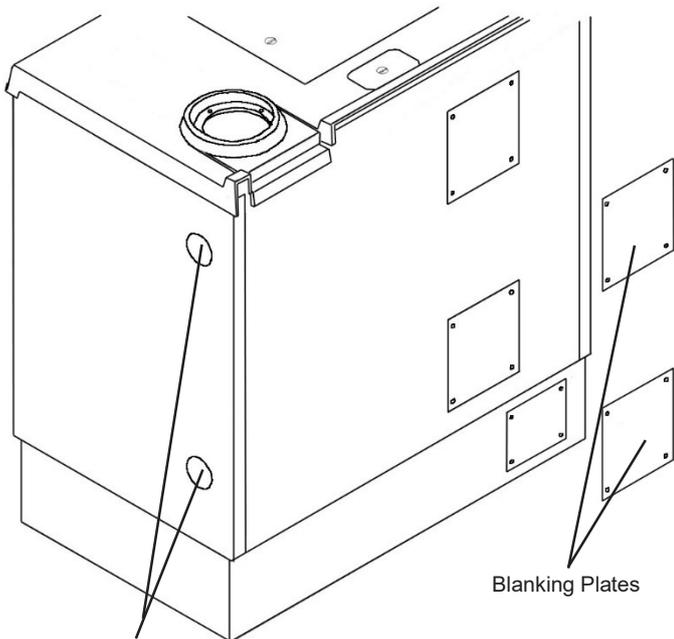
50mm Knockouts RH Boiler Connections
