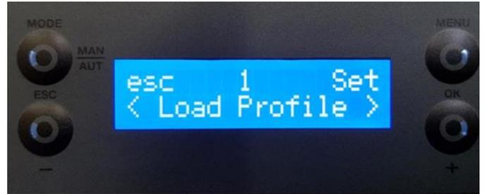
Press the "+" key to go to menu "Reset". This menu allows you to delete any programme settings. To do this, press "set". The "Confirm" appears. Press "set" again to confirm that you want to delete the settings or "esc" to exit.
