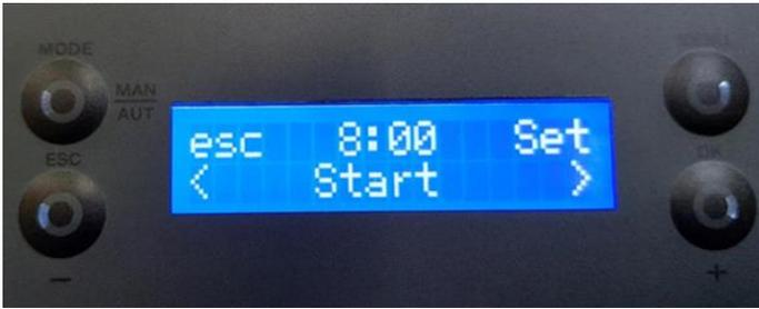
To set the starting time for Programme P1, press "set". The display starts to flash. Press the "+" or "-" key to select the time and then press "ok" to confirm. Press the "+" key to go to the P1 ." Stop" menu.
