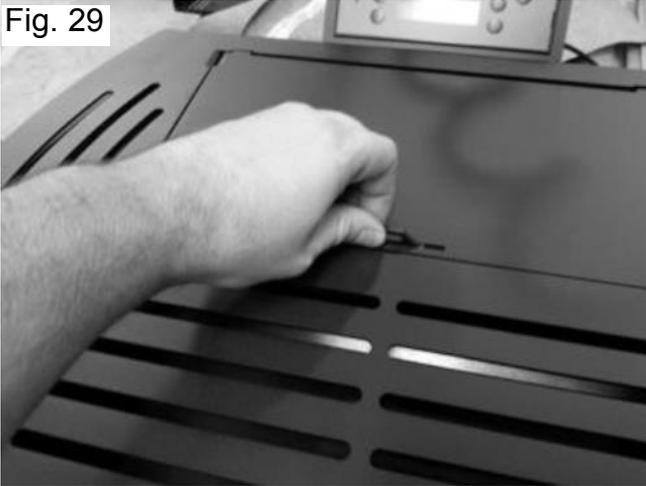
The reservoir will hold approx 15 kg on the K100 with the K300 holding approx 18kg to fill the hopper carefully cut the corner of the bag so the pellets can be poured into the hopper without spilling outside of the rubber seal. Do not pour dust into the hopper as it can impair the feed screw mechanism.
