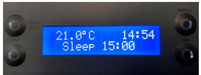
The display will then switch between the normal screen and a screen similar to above showing the current time and the sleep time at which the stove will switch off.
