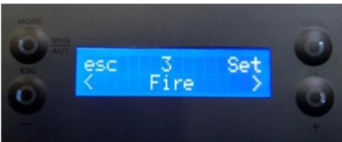
To set the operating power level (1 to 5) of Programme P1, press "Set". The display starts to flash. Press the "+" or "-" key to select the desired power level (1 to 5), and then "Ok" to confirm. Press the "+" key to go to the "Days" menu.
