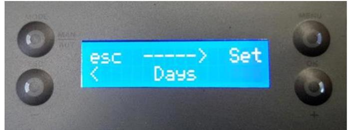
To select the days of the week that you want P1 Programme to run, press "set" and then select the day of the week using the "-" and "+" keys. Press "set". The display starts to flash. Select "On" or "Off" using the "-" and "+" keys. Press "ok" to confirm the selection. Press the "esc" key to go to the "Days" menu. Press the "esc" key again to go to the "program " menu. Press the "+" key to move on to the next menu.
