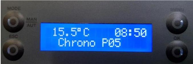
When the unit is set to switch on and off using the programmer the display will flash between the on/ off screen and a screen similar to above.
