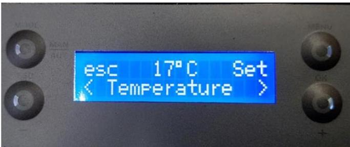
To set the set point temperature for Programme P1, press "Set". The display starts to flash. Press the "+" or "-" key to select the desired temperature, followed by "Ok" to confirm.
