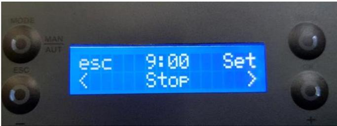
To set the stopping time for Programme P1, press "set". The display starts to flash. Press the "+" or "-" key to select the time and then press "ok" to confirm. Press the "+" key to go to the "Air Temperature "menu.
