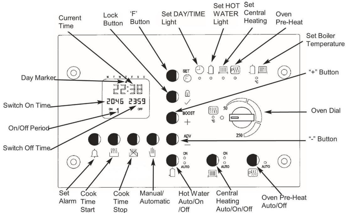
The programmable clock controls your central heating system and oven preheat function, and allows you to set your cooking times automatically. The clock offers the following features:
