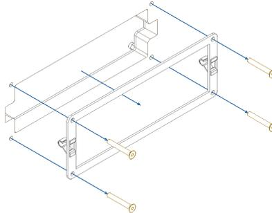
**Figure 16 – Installing the display outside the device**
