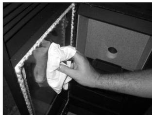
**Figure 46 – Cleaning the glass: Cleaning the glass with the cloth**
