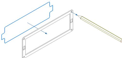
**Figure 14 – Installing the display outside the device**
