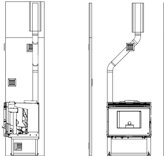
Figure 41 - View installation with chimney.
