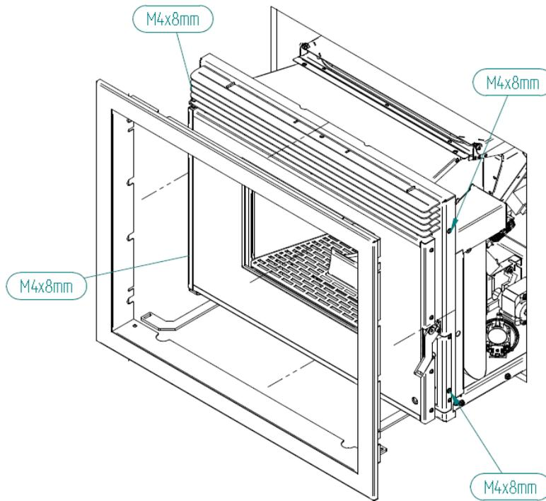
**Figure 35 - Locating the screws to attach the frame to the insert**
