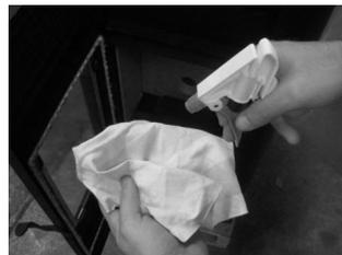
**Figure 45 – Cleaning the glass: Applying liquid to the cloth**
