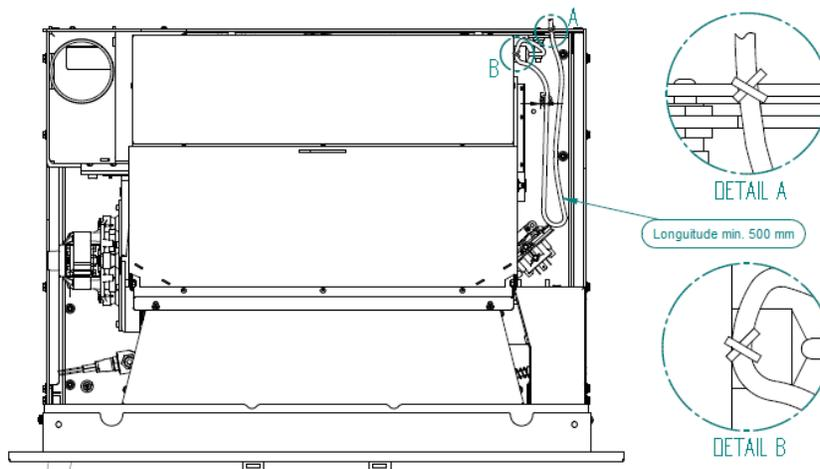
Figure 32 – Electrical connection plug
