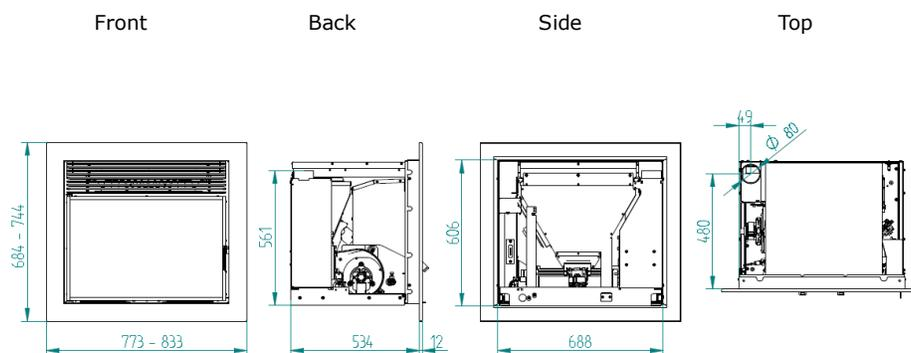
**Figure 4 – Insertable dimensions to pellets**
