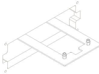
**Figure 15 – Installing the display outside the device**
