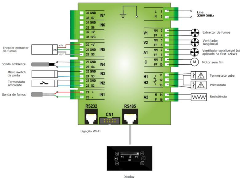
Figure 53 – Electrical diagram (Tiemme Electronics)
