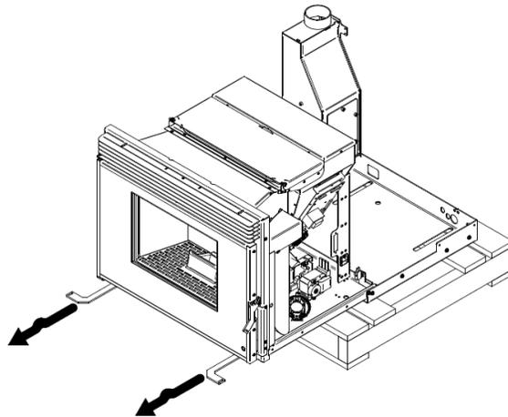
**Figure 2 – Separate moving and fixed parts**
