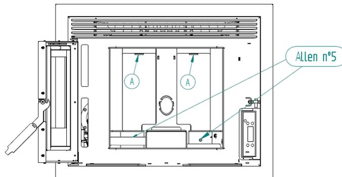
**Figure 42 – Combustion chamber separators**
