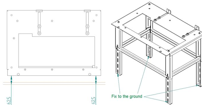
**Figure 29 – Auxiliary table assembly**
