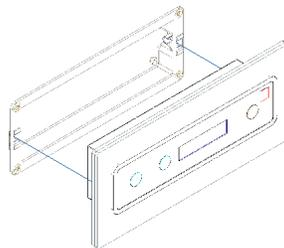
**Figure 17 – Installing the display outside the device**
