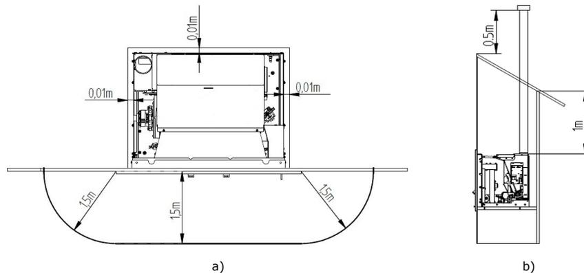
**Figure 31 – Minimum distances of all surfaces: a) top view of the installation of the equipment; b) side view of the equipment installation**
