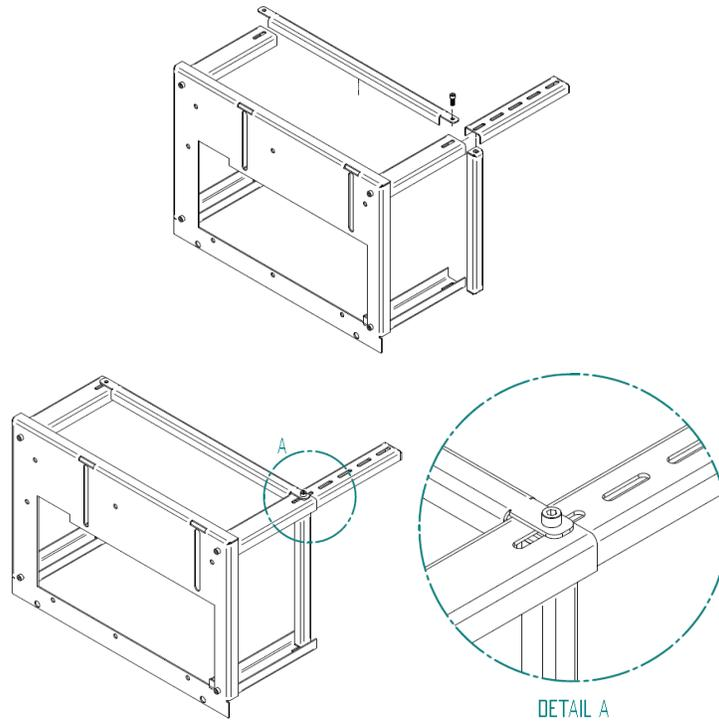
**Figure 26 – Auxiliary table assembly**
