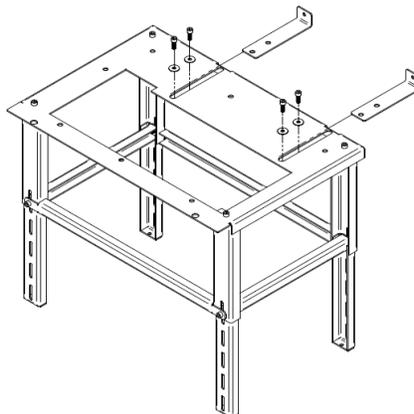
**Figure 28 – Auxiliary table assembly**
