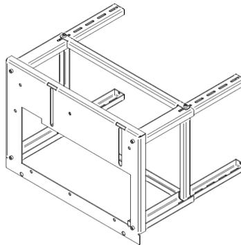
**Figure 27 – Auxiliary table assembly**
