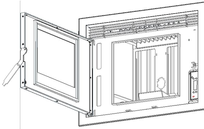
**Figure 43 – Fume passage cleaning and cast-iron heat exchanger**
