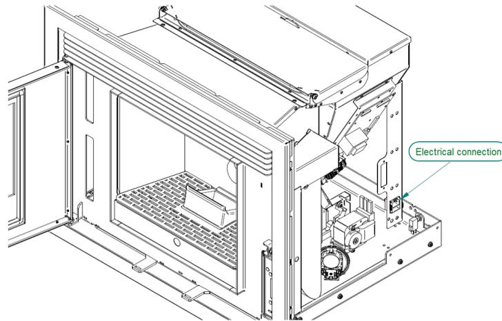
**Figure 10 – Electrical connection**
