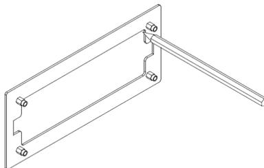
**Figure 13 – Installing the display outside the insert**
