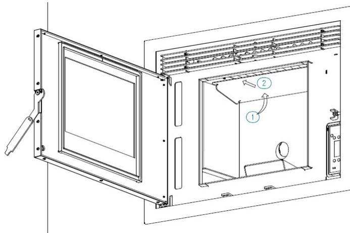
**Figure 41 – Removal of the baffle plate**
