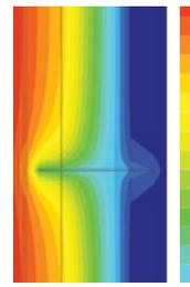
Insulation performance is no longer about simple U-values. How that insulation interconnects with other elements and junctions in the design is critical. The aim is to achieve a continuous thermal layer that minimises heat loss at those junctions. This is thermal bridging and is measured and
