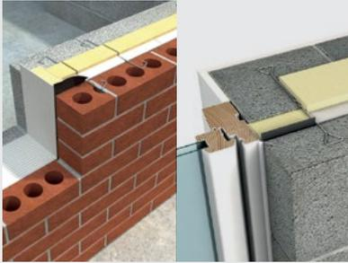
15 In accordance with S.R. 325 a vertical DPC should be provided that extends 25mm beyond the width of the closer.
