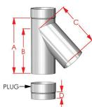
A 45° Tee is used to create a bend in a flue run. It can be used to change a chimnev from run horizontal to a vertical run when used with a 45° bend. This component minimises resistance to the the angle because of created with the vertical component axis. This comes complete with a removable inspection cap.
