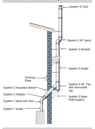
System 1 used as Rigid Flue Liner
