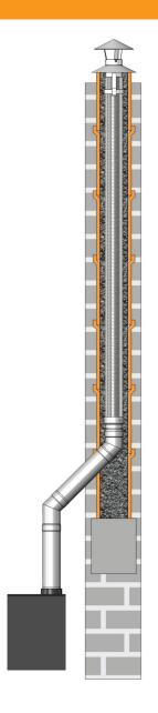
**Single Wall Connecting** Flue Pipe for Multi-Fuel **Appliances**
