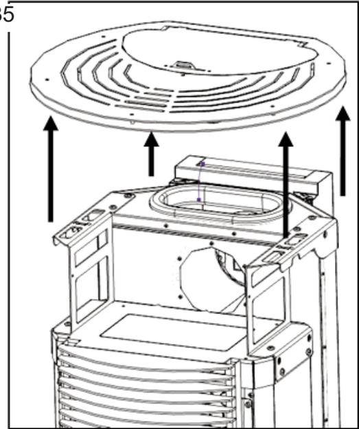
Place the upper front as shown in the picture below, the flaps of the upper front must go inside the frame of the stove.
