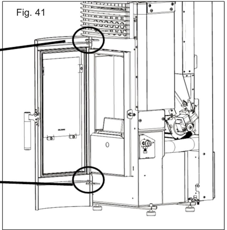
To fit the side panels it is necessary to remove the door from the stove, to remove the door, open the door first, lift the door to allow the bottom pin to disengage, move the door slightly to allow the door to drop without re-engaging the bottom pin then lower the door gently
