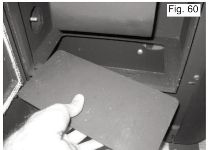
When the area is cleaned replace the trapdoor making sure it is seated correctly.
