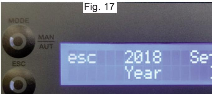
To set the year press "set". The display starts to flash. Press the "+" or "-" key to select the desired year and then "ok" to confirm.
