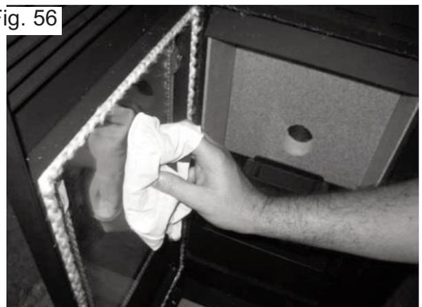
Fig.65 & 66 – Correct cleaning of the glass.
