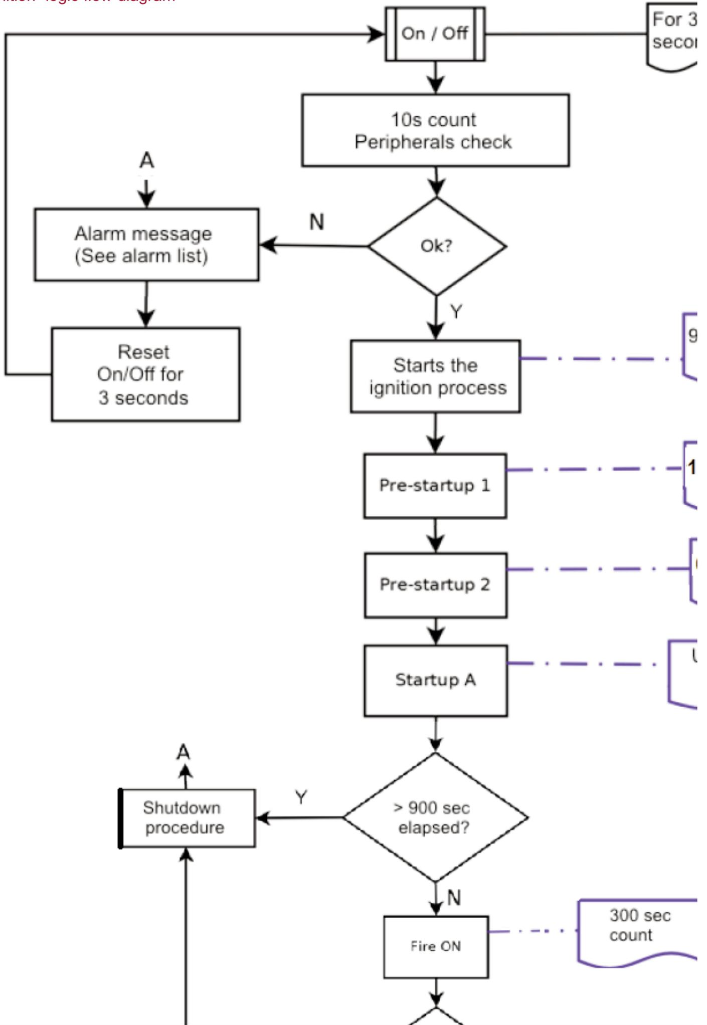
Shut down logic flow diagram
