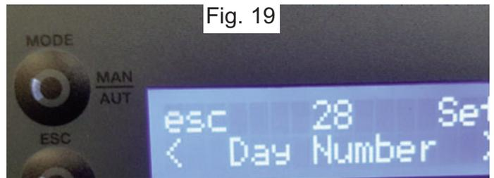
To set the "Date" press "set". The display starts to flash. Press the "+" or "-" key to select the desired date and then "ok" to confirm
