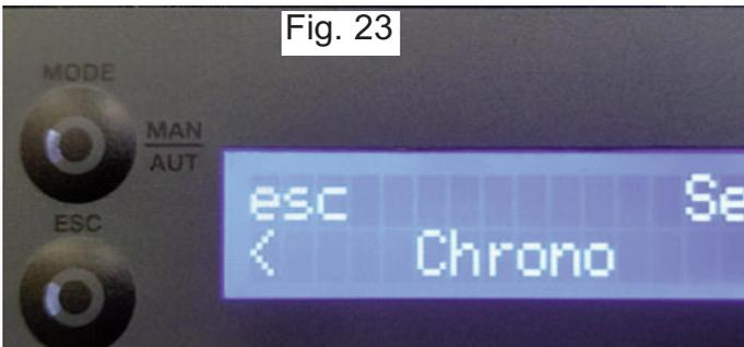
To activate the Timer mode, press "Set" the display starts to flash. Press the "+" or "-" key to select "On" or "Off" and then "Ok" to confirm. Press the "+" key to scroll to the "Load profile" menu.
