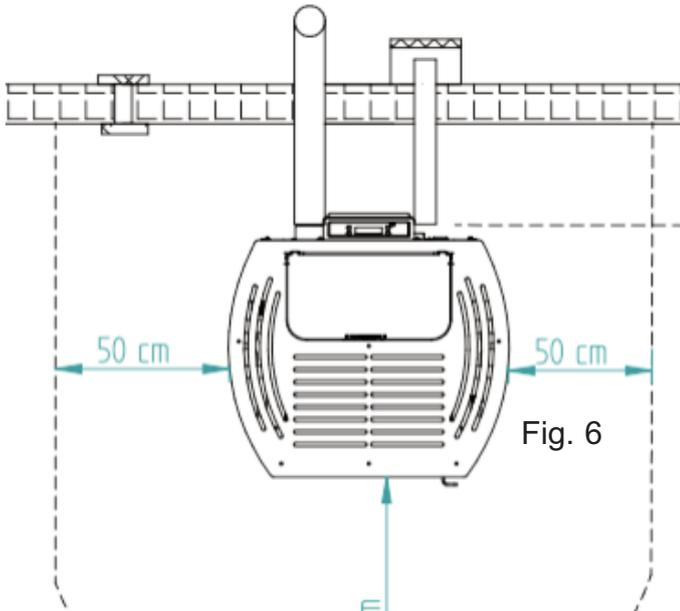
In the event that the product is installed in a non combustible recess, clearances for servicing, must be provided, 200mm to the rear and 300mm to the sides.
