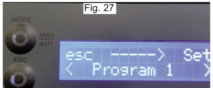
Press "Set" again and when the display starts to flash, press the "+" or "-" keys to select "On" or "Off". Press "ok" to confirm the selection. Press the "+" key to go to the "start" time.
