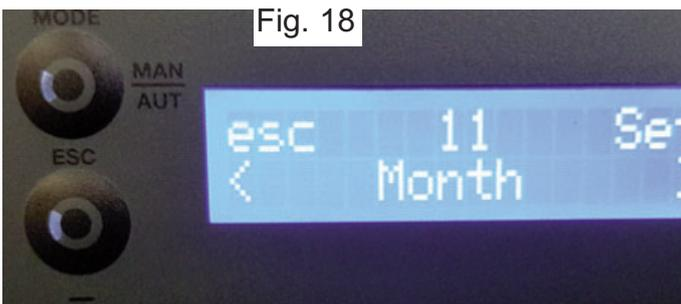
To set the "month" press "set". The display starts to flash. Press the "+" or "-" key to select the desired month and then "ok" to confirm
