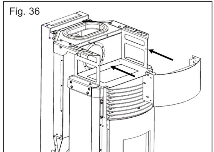
Screw the upper front to the frame using two of the screws provided. Place screws in the location shown below. Do not fully tighten as a small adjustment may be necessary.
