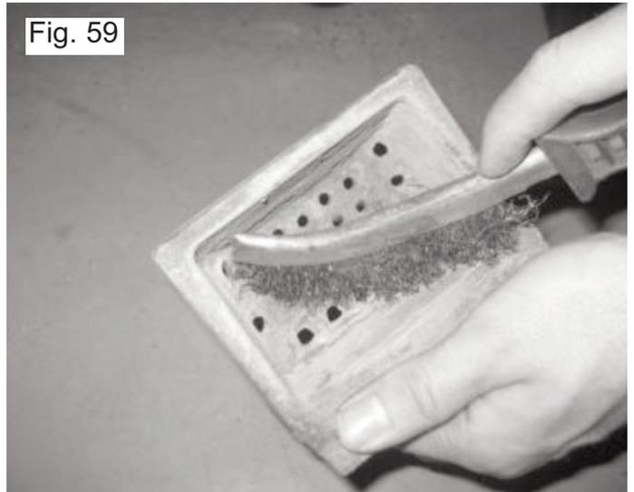
Put the burnpot back in place, making sure that it is seated properly, if the burnpot is seated incorrectly it will lead to problems during ignition or poor performance.
