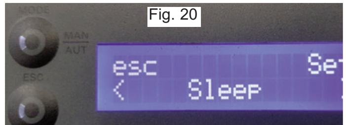
Press "set". The display starts to flash. Select the desired time using the "-" and "+" keys. After choosing the time, press "ok" to confirm. Press " esc" when finished to get back to the normal display
