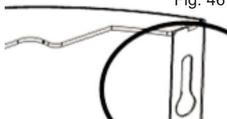
When fitting the covers, check that the tabs on the bottom overlap the combustion chamber and that the upper parts rest on the structure of the equipment
