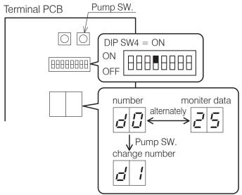
Figure 10-2: Display on Terminal PCB display
