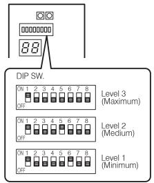
Figure 8-9: Pump output adjustment flow rate - DIP switches
