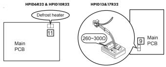
Figure 11-8: Resistance of the defrost heater
