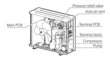
Figure 1-4: Main components (internal) - 6kW
