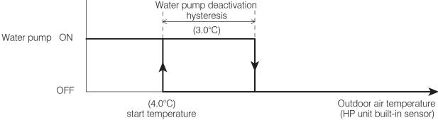
Figure 8-16: Frost protection (outdoor air temperature) - water pump
