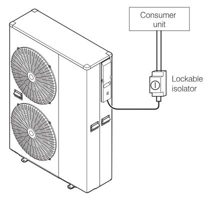
Figure 6-4: Heat pump, isolator and consumer unit
