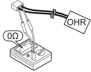
Figure 11-10: Resistance of the compressor overheat protection relay
