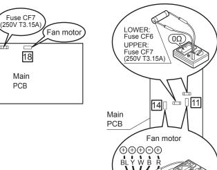
Figure 11-4: Voltage of Fan motor on the Main PCB
