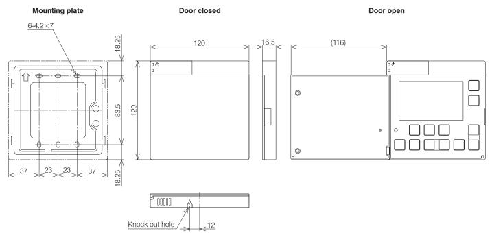
Figure 2-6: Remote controller dimensions
