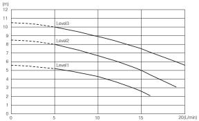
Figure 8-10: Pump output adjustment flow rate - HPID6R32
