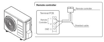
Figure 7-6: Connecting the display pad to the heat pump
