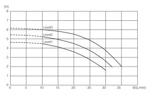
Figure 8-11: Pump output adjustment flow rate - HPID10R32
