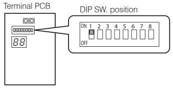
Figure 3-8: Anti-freeze function setting
