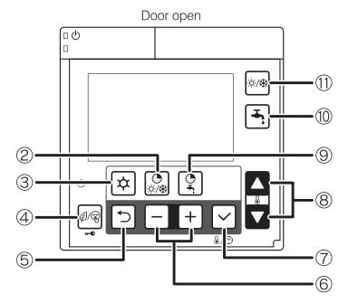
Figure 10-1: Remote controller buttons
