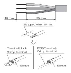
Figure 6-5: Stripping the cables
