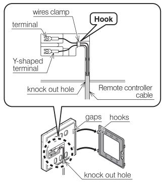
Figure 7-5: Connecting display pad cable
