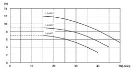
Figure 8-13: Pump output adjustment flow rate - HPID17R32
