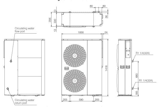
Figure 2-5: HPID13R32 & HPID17R32 dimensions
