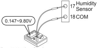
Figure 11-11: Voltage of humidity sensor
