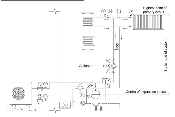
Figure 3-4: Monovalent system - with S-Plan type controls
