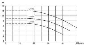
Figure 8-12: Pump output adjustment flow rate - HPID13R32
