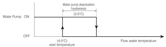
Figure 8-17: Frost protection (flow water temperature) - water pump
