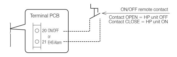
Figure 8-21: ON/OFF heating remote contact
