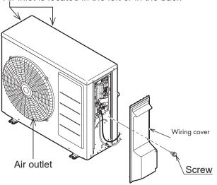
Figure 1-1: Main components (external) - 6kW
