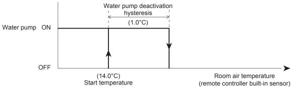
Figure 8-18: Frost protection (room air temperature) - water pump
