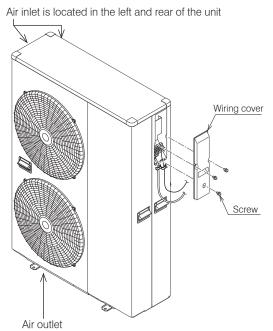
Figure 1-3: Main components (external) - 13kW & 17kW
