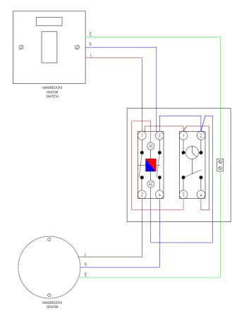
Figure 5-4: Boost kit wiring diagram
