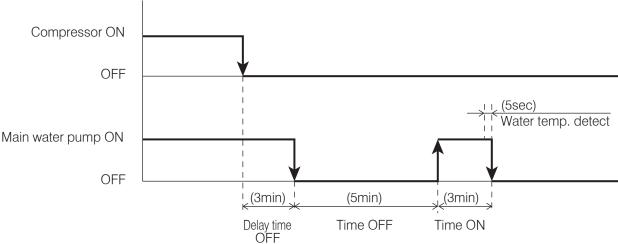
Figure 8-6: Detect cycle
