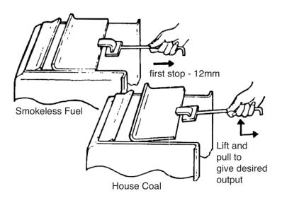
A deepening bar should be fitted when burning smokeless fuels and removed when burning coal.
