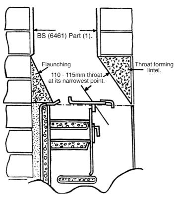
A throat-forming lintel should be installed, leaving an opening of approximately 110mm between boiler and lintel (not to exceed 115mm, see diagram). The sides and back must lead with a gradual slope up to the start of the flueway at an angle not more than 30° to the vertical - rendering may be necessary to achieve these conditions.
