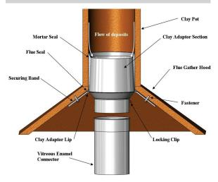
To install Mi-Flues Clay Adaptor, place a bead of Mi-Flues high temperature sealant (rated to 1000°C) or a suitable flue seal around the clay adaptor lip on the side to mate with the clay pot<sup>\*</sup>.
