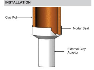
In order to install an Mi-Flues External Clay Adaptor, slide the clay adaptor over the clay pot. Once placed into position, seal the cavity between clay pot and adaptor using mortar.
