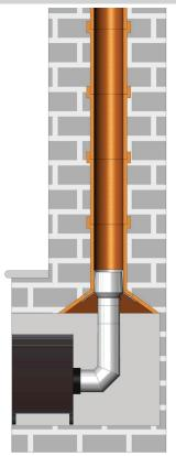
Mi-Flues Clay Adaptor kits can only be used when cleaning and removal access is provided directly through the appliance.
