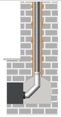
Mi-Flues Insert Stove kits can only be used when cleaning and removal access is provided directly through the appliance.
